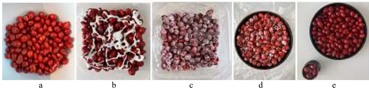
Figure 3 – Preparation steps of Material I: a) Painted cherry seeds b) Addition of tree glue c) Mixing tree glue and red cherry seeds d) The prepared mixture in the mold e) Mixture upon drying
